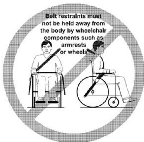
Belt restraints should make full contact with the shoulder, chest, and pelvis and pelvic belts should be positioned low on the pelvis near the thigh-abdominal junction.
